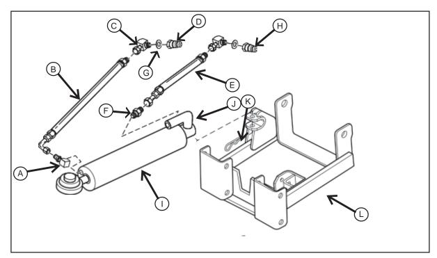
Figure 2. Cylinder/Hose Installation
